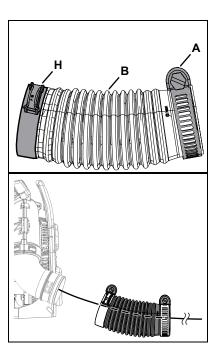
3. Assemble flexible pipe to elbow (D) on blower. Position clamp with cable guide loop (H) on outside of flexible pipe and tighten clamp.
