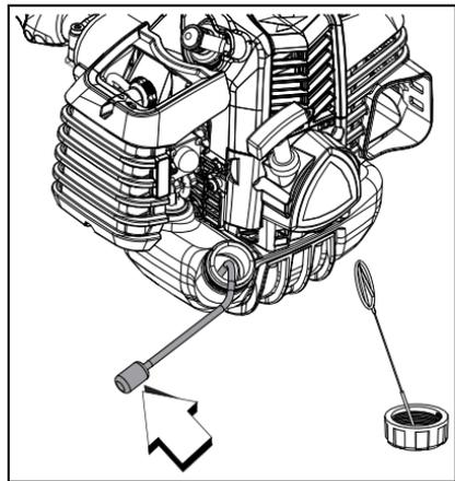
Note: Federal EPA regulations require all model year 2012 and later gasoline powered engines produced for sale in the United States to be equipped with a special low permeation fuel supply hose between the carburetor and fuel tank. When servicing model year 2012 and later equipment, only fuel supply hoses certified by EPA can be used to replace the original equipment supply hose. Fines up to \$37,500 may be enforced for using an un-certified replacement part.
