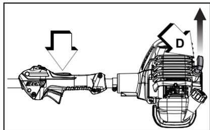
Note: If engine does not start with choke in “RUN” position after five pulls, repeat instructions 2 - 5.
