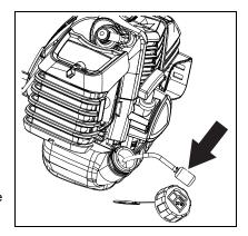
6. When the inside of the fuel tank is dirty, rinse the tank out with gasoline to clean it.
