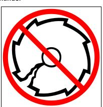
When sharpening a blade, always remove the same amount of materials from each tooth to maintain balance. A blade that is not balanced will cause unsafe handling due to vibration and can result in blade failure.
