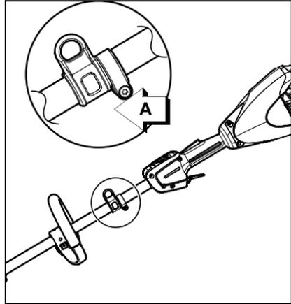
3. Slide harness clamp up or down until unit balances with head or blade  $200\text{ mm} \pm 100\text{ mm}$  ( $8\text{ in} \pm 4\text{ in}$ ) from the ground.
