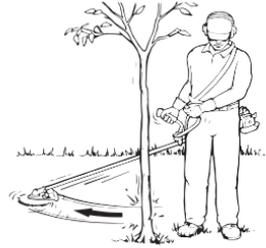
To free a blade that is bound in the cut, stop the unit, and support the trimmer or brushcutter to keep stress off the blade. Push the tree away from the entry point of the cut to open the cut, and pull the blade directly away from the cut in a straight-line motion. Use caution when releasing the tree to avoid being struck by spring-back or falling.
