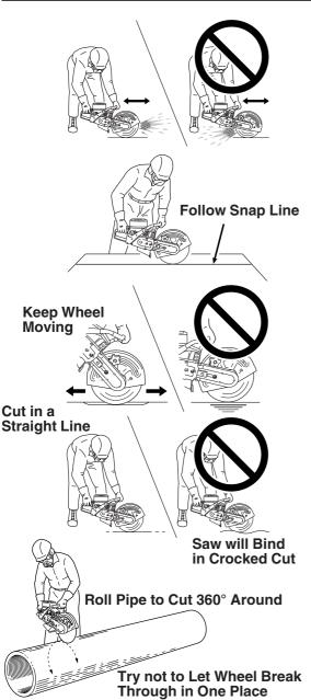
The main objectives are to avoid overheating the wheel, and to prevent it from being pinched or trapped or stressed in any way.
