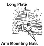
When necessary to cut up close to a barrier, invert and remount the arm so the wheel is on the outboard side.
