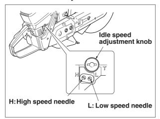
Every unit is run at the factory and the carburettor is set in compliance with Emission Regulations. In addition, the carburettor is equipped with "H" (High Speed Needle) and "L" (Low Speed Needle) needle adjustment limiters that prevent settings outside acceptable limits.
