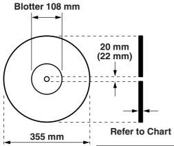
Wheel blotters attached to both sides of reinforced wheels are cushions needed to equalize the pressure of the mounting flanges from wear if slippage between the wheel and the flanges occurs. The blotters are 108 mm diameter. Take care that the blotters do not become gouged or deeply scratched and that there is no foreign material on them when mounting the wheel.
