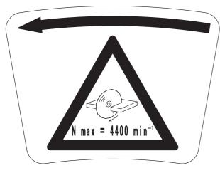
Maximum wheel speed is indicated. Wheel rotation direction is shown by arrow.
