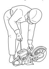
Set saw down on level ground with wheel or saw blade in the clear. Grasp front handle with left hand, and hold down rear handle with toe of your boot. Never "drop-start" the saw.
