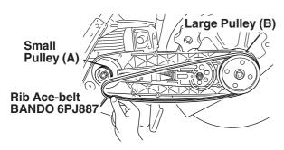
Push arm towards small pulley. Pull belt off pulley at point (B) and slip new belt onto small pulley. At point (A), start belt over the rim and onto the large pulley.
