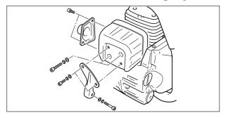
The dust created in cutting is drawn into the cooling system by the rotor fan. It can cover the cooling fins and clog the air passages. Unless the system is cleaned in time, the engine will run too hot. Whenever cleaning the cooling system, take advantage of the necessary removal of the covers, and check the muffler at the same time.
