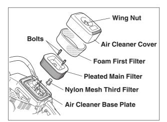
Dust from cutting must be prevented from entering the engine. The three (3) filters in the Air Cleaner System can do this if they are properly maintained and correctly installed. The foam, first filter when used dry should be removed and cleaned each time the fuel tank is refilled. If the foam filter is oiled [recommended to prolong main (paper) filter life], cleaning may be required more frequently if a noticeable drop in power due to a clogged air filter is noted.
