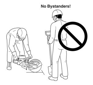
Spectators children and fellow workers must be warned to come no nearer than 9 m while the saw is in use. Shut off the saw immediately if some one moves closer to you than 9 m. Persons working in the area near you should wear the same protective equipment as the saw operator if endangered by risky flying debris.
