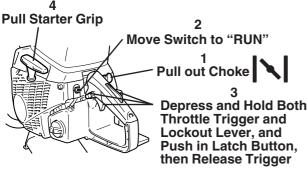
6 To De-latch Throttle, Squeeze and Release the Trigger
