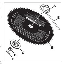
Never reuse a cotter pin. Install a new cotter pin each time a blade is installed or replaced.
