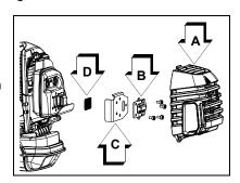
Note: When cleaning carbon deposit, be careful not to damage the catalytic element inside muffler.
