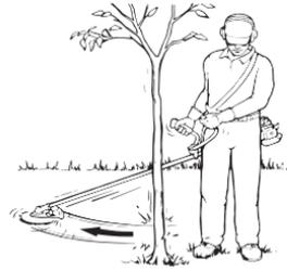
To free a blade that is bound in the cut, stop the engine, and support the trimmer or brushcutter to keep stress off the blade. Push the tree away from the entry point of the cut to open the cut, and pull the blade directly away from the cut in a straight-line motion. Use caution when releasing the tree to avoid being struck by spring-back or falling.
