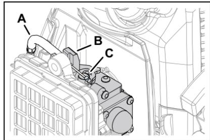
Note: The throttle linkage must be adjusted by moving the adjustment nut. Consult with your Authorized Service Dealer for correct adjustment procedure.
