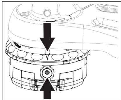
3. Insert one end of trimmer line into an eyelet, and push line equal distance through trimmer head.
