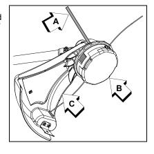
Retain line head, shield plate, and shield with cut-off knife for conversion back to nylon line head operation. ASSEMBLY SRM-2620U
