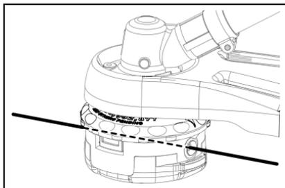
4. Hold trimmer head while turning knob clockwise to wind line onto spool until about 130 mm (5 in.) of each line remains exposed.
