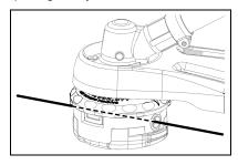
4. Hold trimmer head while turning knob clockwise to wind line onto spool until about 13 cm (5 in.) of each line remains exposed.
