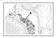
Note: The throttle linkage must be adjusted by moving the adjustment nut. Consult with your Authorized Service Dealer for correct adjustment procedure.
