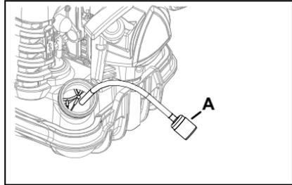
Note: Federal EPA regulations require all model year 2012 and later gasoline powered engines produced for sale in the United States to be equipped with a special low permeation fuel supply hose between the carburetor and fuel tank. When servicing model year 2012 and later equipment, only fuel supply hoses certified by EPA can be used to replace the original equipment supply hose. Fines up to \$37,500 may be enforced for using a replacement part that is not certified.
