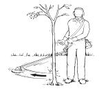
To free a blade that is bound in the cut, stop the unit, and support the trimmer or brushcutter to
