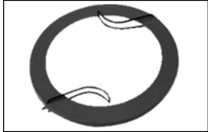
Use blade protectors to protect blade teeth during unit transportation.
