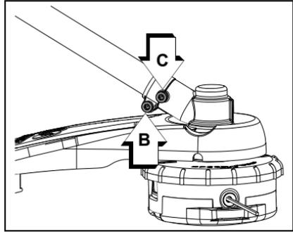
2. Pull flexible cable (D) from the drive shaft housing, wipe clean and coat with 15 ml (0.5 oz.) of grease.
