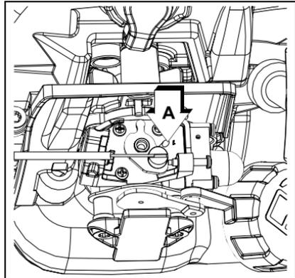
2. Remove air filter cover. Brush dirt from inside cover.
